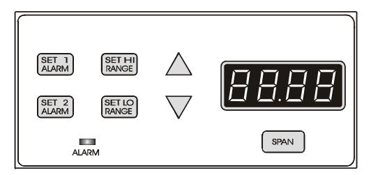
Figure 4-1: Front Panel Controls and Indicators
